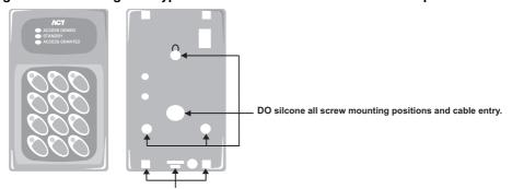
DO NOT apply silicone to the bottom of the keypad as this will block the air vents and trap any water which may enter the keypad If a weather shield is fitted the same applies
